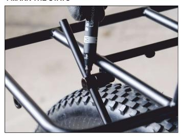
Mark the stays aca 10mm over where they exit the eyebolt drilling. Take the stays off the rack and cut them where you marked them. File or sand the stay ends and remove all burs or sharp edges.
