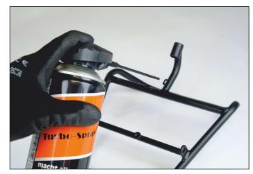
If you live in very moist and wet areas, especially close to the sea, we recommend to use some spray lubricant like WD40, Fluidfilm, Mike Sanders, etc inside the rack. Spray a small amount inside every venthole at the backside of the rack before installation. Move the rack around and let excess oil come out of the ventholes. You can also oil the hardware parts such as bolts and lightmount in order to prevent them from rusting. **Make sure there is no oil dripping on your brakes and discs!!**
