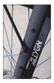
Install the rack stays loosely to the rack as shown on the illustration on page 2. Then mount the stays to the midfork eyelets. Fasten the screws loosely at this point, so you can still adjust the rack angle at this point.
