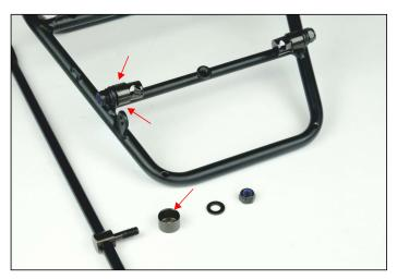
We found out that some people seem to forget to install the stepped washers on top of the eyebolts. It is very important to install those parts correctly, otherwise the rack stays will not carry the load and the rack will not be safe to use !!!
