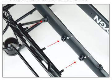
If you want to use anything cages mounted on top of the racks stays, then please use the included 12 x 5 x 5mm plastic spacers to make up for the rack stays thickness.
