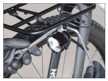
If you have a frontlight which can be mounted upside down then just mount it to the light tab on rack using the M6 x 22mm bolt, washers and nuts.
