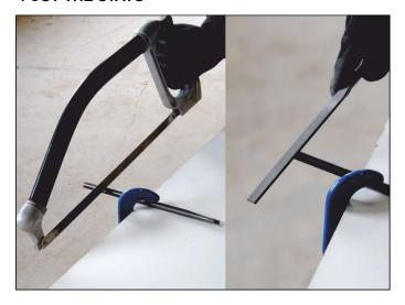
After cutting the stays repeat steps 1 - 3 and use Loctite 243 for mounting the M6 fork crown bolt and M5 bolts to the forkleg lowrider mounts.
