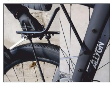
Install the rack stays loosely to the rack as shown on the illustration on page 2. Then mount the stays to the midfork eyelets. Fasten the screws loosely at this point, so you can still adjust the rack angle at this point.
