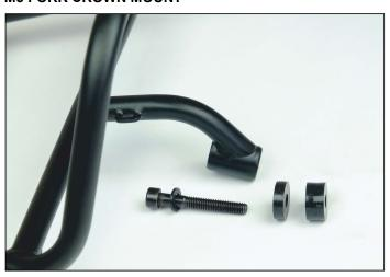
If your fork has an M5 fork crown mount then use the M5 bolt and washer. If needed, use one or more spacers and select the right length of bolt. Please use Loctite 243 medium tight or similar!
