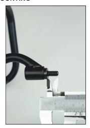
On carbon forks the mounting points are sometimes deadend threads so it is very important not to use bolts that are too long as this can result in damaging the mounting point and / or the fork itself. Measure how far the thread goes inside and select the length of bolt accordingly!
