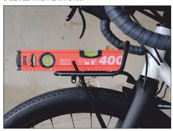
Check in side view if the rack is level to the ground. Use an spirit level if you have one. Adjust the rack angle in front view and check if it's level relative to the headtube. Check side view again and re-adjust if necessary.
