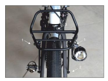
Gently tighten eyebolts on rack (1) first. Then tighten the stays to the mid forkleg lowrider mounts alternating left and right (2). Finally tighten the M6 to the fork crown (3). Double check again if the rack is really level in both views. Re-adjust if necessary.
