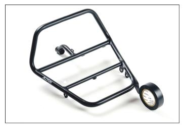
We deliberately chose a hard wearing coating for the racks, but it is still just paint and if used hard it will wear off, there is no way to avoid that! You could use electrical tape or (even better) 3M helicopter tape in order to protect the racks paint. If the paint wears off and you see blank metal, no worries, just use a little bit of oil to prevent it from rusting. Light surface rust will not seriously damage the rack!
