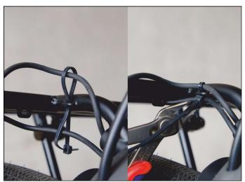
Put the zip ties in a figure 8 through the racks cable tabs. Run the cables left and right to the tabs. Do not tighten the zip ties yet! Arrange all cables neatly and make sure you have enough cable for frontlight adjustment. Finally secure the zip ties and cut the ends.
