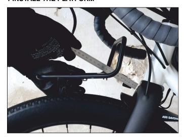
Place the front rack centererd over the front wheel. Measure the distance between fork crown mount and rack and select spacers accordingly.
