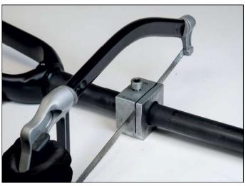
Use a saw guide to make a straight cut. Never freestyle cut just by hand! Cut all the way through and make sure not to damage the fibers. Use sandpaper to smooth the cutting edge / outstanding fibers. Use a face mask to prevent you from breathing in saw dust and fibers!
