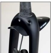
The fender stays can be attached to the lower fork leg M5 eyelets (5 Nm). Always use Loctite on all fender bolts and frequently check that all bolts are tight! **Fender to tire minimum internal distance must be at least 15 mm!** Don't forget to tighten down the fork wheel axle with 9-13 Nm before you go on your first ride!
