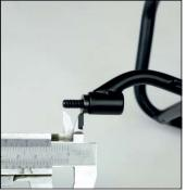
The fork crown mount is a 12 mm deep blind hole so it's very important not to use too long bolts, as this can result in damaging the threads and/or the fork itself. Measure how far the thread goes inside and select the right length of bolt accordingly! Max load for the fork crown bolt is 3 kg, maximum torque is 6 Nm. Always use Loctite and check regular if the bolt is still tight!
