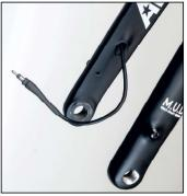
Punch a hole or cut a slot into the rubber grommet and pull the cabel through the seal. Make sure you have at least 10 cm extra cable length sticking out the bottom cable port before soldering the connectors. Excess cable can easily be stuffed back inside the fork leg and will be very helpful to prevent ripped off dynamo cables.
