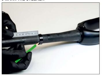
Make sure the fork is all the way inserted in the frame and the headset / stem / spacers are all compressed nicely. Use a sharp pencil to mark the steerer at the top spacer (refer to picture 2). Take the fork out of the frame and mark the final cut 4-5 mm lower then your top pencil marking (this picture).
