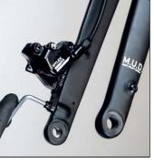
Route the brake hose through the inner brake cable routing. Install the brake flat mount adapter to the lower left fork leg brake mount. Tighten down the bolts with 6 Nm. Use Loctite, check regular if bolts are still tight.
