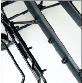
You can install anything cages or racks to the 3 fork leg mounts. Maximum load per bolt is 2 kg, resulting in a maximum load of 6 kg per side if you use all three bolts. Maximum torque is 5 Nm, use Loctite and check regular if the bolts are tight. Do not overtorque, don't screw in at an angle, the fork leg threads can easily be damaged!
