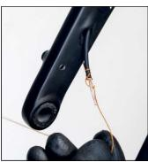
Install your front light to the fork crown. Fasten your light-to-dynamo cable to the pull string and pull the cable through the right fork leg. ( Pro Tip: you can easily re-thread the pull string through the fork leg again using a vacuum cleaner )
