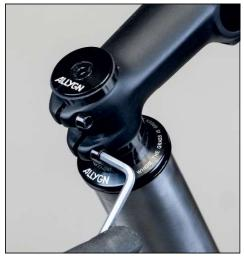
Install the included fork steerer expander. Tighten down the center bolt with max 9.5 Nm. Put the stem (do not tighten the stem clamping yet!) and spacers back on, make sure you still have some space (minimum 2 mm) between the expander top and under the top cap, allowing you to tighten
