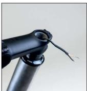
Route the tail light cable underneath the fork crown through the left cable groove. Fix the cable with the 25 mm washer and the flat top cap torx bolt. Use Loctite.
