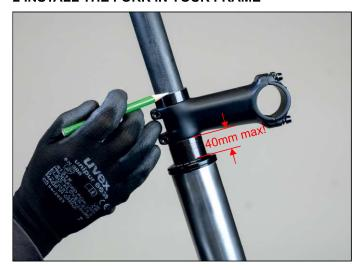
Install the fork in your frame, with the actual headset, all spacers and the stem, just the way as you want to ride your bike later. Maximum spacer height is 40 mm under the stem. If you are unsure about the final stem / handlebar hight, use one or two spacer more and maybe put 1-2 cm spacers on top of the the stem. You can always cut the steerer shorter later.
