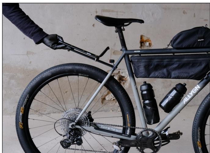
Mount the rack loosely to the rear of the bike. Check which angle and distance to the seat tube best suit your needs. The rack should be mounted as close to the seat tube as possible, but make sure that your inner thighs do not touch when the rack is loaded.
