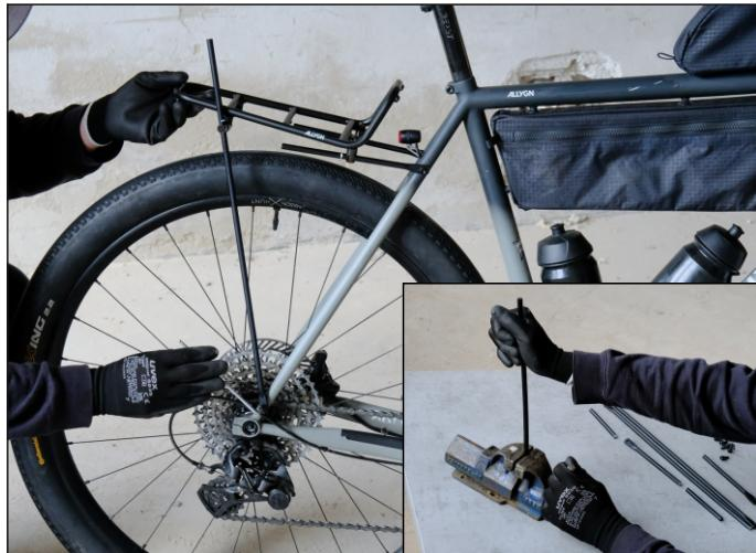
Install the long rear stays on both sides. Gently tighten all nuts and bolts.
