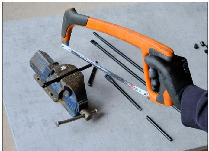
Cut all stays to the correct length. File or sand the stay ends and remove any burrs or sharp edges.
