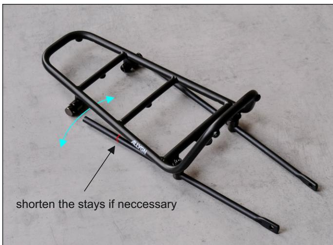
Preinstall the short rack stays at the rear of the rack. If the rack is positioned close to the seat tube, it may be necessary to roughly cut the stays so they can rotate freely during installation without interfering with the rear stay mounts.
