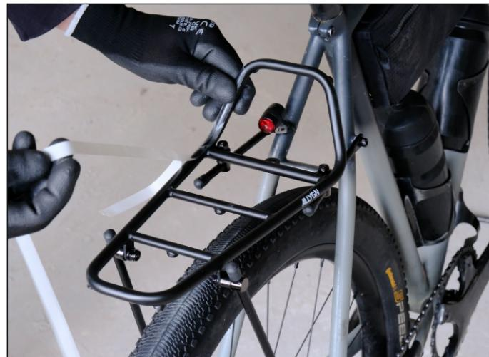
We deliberately chose a hard-wearing coating for the rack, but it will wear over time with use. Our optional 10 mm 3M Helitape strip is ideal for protecting the rack tubes from wear. Alternatively, gaffer tape or electrical tape can be used. If the paint is damaged and bare metal becomes visible, simply apply a small amount of oil to prevent rust. Light surface rust will not seriously damage the rack.
