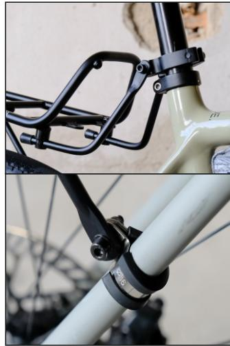
If your frame does not have mounts on the seat stays or dropouts, you can use our optional P-clamps. Always use protective tape to protect the bike frame. Don't use the P-Clamps on carbon frames, they may destroy your frame.
