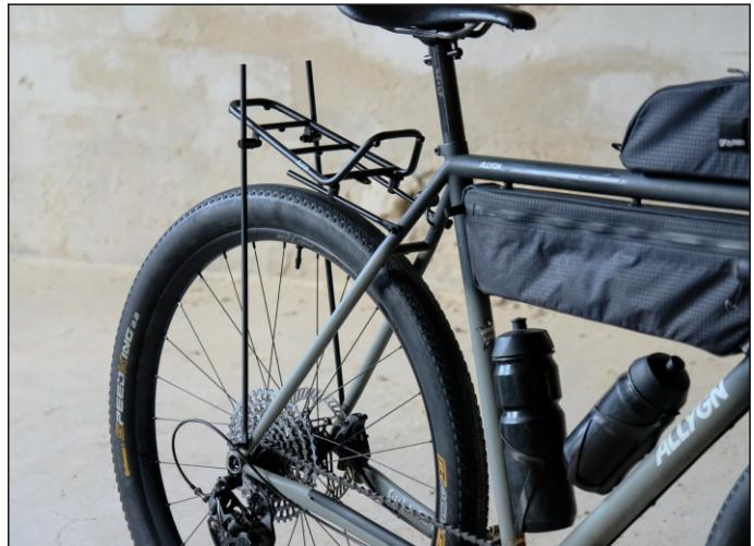
Step back and check all angles. Make sure the rack is centered nicely over the tire.
