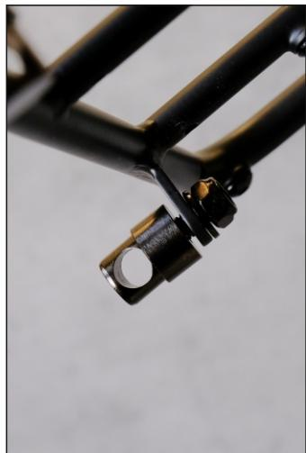
The eyebolts must be installed like this:
