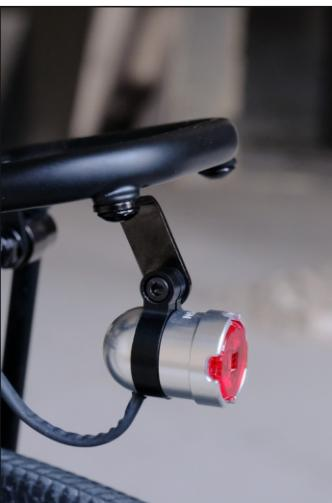
Taillights with 50 mm mounting spacing can be attached using the optional Taillight Mounting Kit. Other lights, such as the EdelMü, can be mounted using a single L-bracket rotated 90 degrees.
