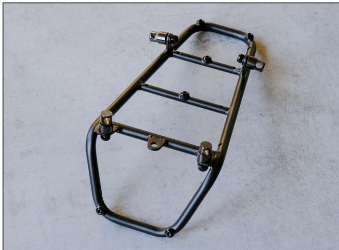
Loosely install all four M6 eyebolts on the rack. Ensure they are mounted as shown in the picture above (bottom view).
