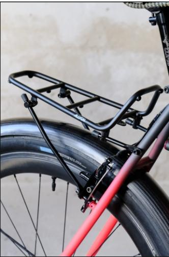
You can use the rack's center mount if your frame only has a single bridge eyelet. Canti studs can also be used for mounting. The aluminum rack stays can be bent for more complicated mounting situations. Bend them slowly and avoid repeated bending, as this may cause them to break.
