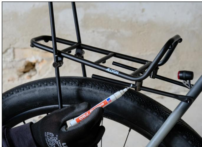
Once you are sure the rack is in the perfect position, mark the stays approximately 14 mm behind the eyebolt. Then disassemble the rack stays again.
